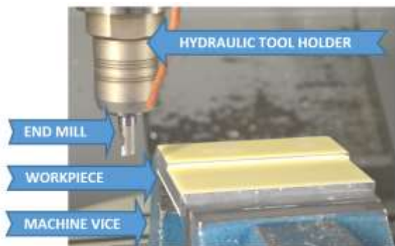
Figure 7. Schema of machining process
