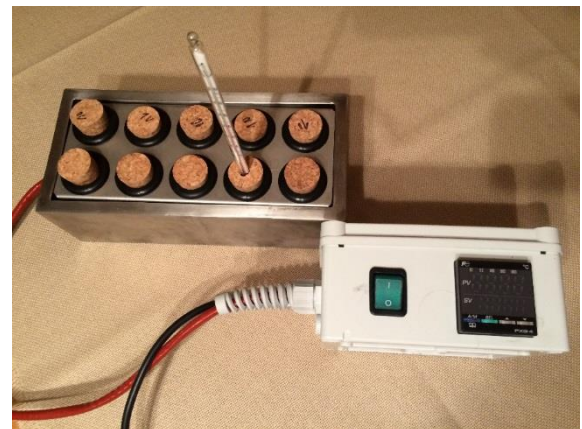
Figure 3. Equipment for the extraction the binders
