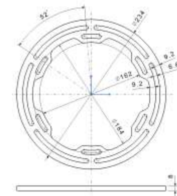
Figure 16. Version 3 – the main dimensions of the composite ring
