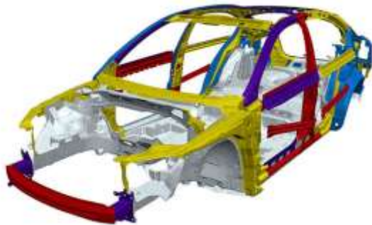
Figure 2: Location of deformation zones on the bodywork
