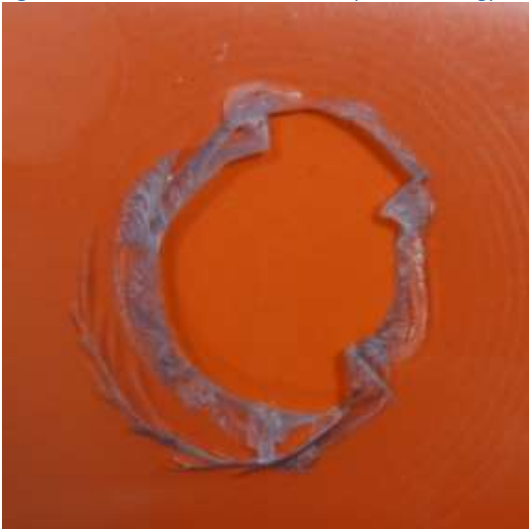
Figure 6: SAN failure after the test at set potential energy 30 J
