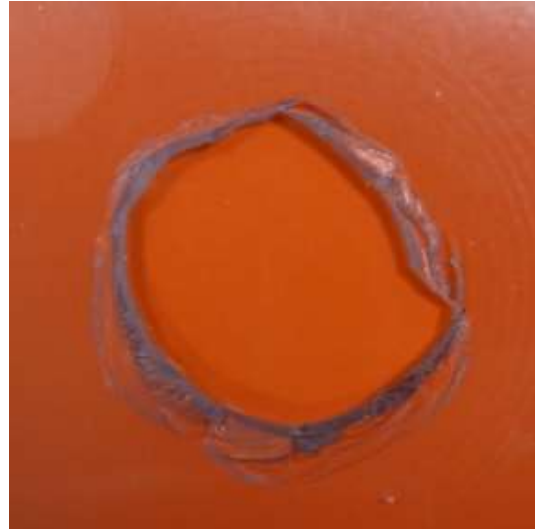
Figure 8: SAN failure after the test at set potential energy 50 J
