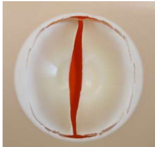
Figure 7: ABS failure after the test at set potential energy 50 J
