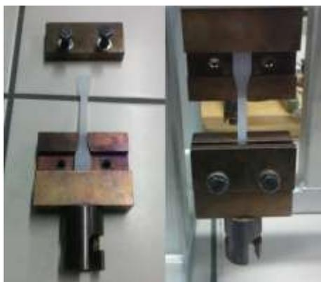
Figure 3: Clamping of sample
