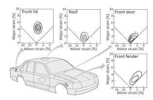
Figure 2. Strain schemes at car-body parts production
