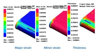
Figure 7. Strains calculated by numerical simulation when bending to  $180^\circ$  – critical major/minor strains [0.07; 0.0007]
