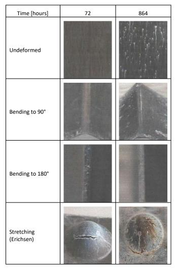
Figure 13. Surface of samples GA2 with Zn-Al-Mg coating after 72 and 864 hours spent in corrosion atmosphere
