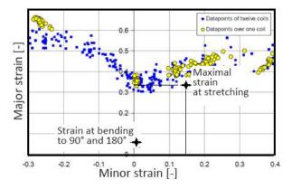
Figure 4. Strains shown in the Forming Limit Diagram for base material DX54D
