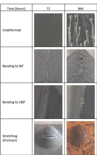
Figure 11. Surface of samples GA1 with Zn-Al-Mg coating after 72 and 364 hours spent in corrosion atmosphere
