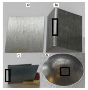
**Figure 3.** The specimens shape after plastic deformation a) no deformation, b) bending 90°, c) bending 180°, d) stretching by Erichsen test
