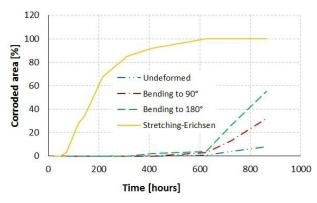
Figure 10. Corroded surface-Time dependence for GA1 samples with Zn-Al-Mg coating
