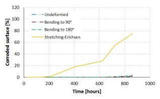
Figure 12. Corroded surface-Time dependence for GA2 samples with Zn-Al-Mg coating
