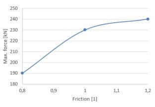
Figure 16. Maximal achieved force of cross wedge rolling with respect to friction
