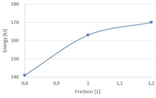
Figure 15. Amount of energy consumption of cross wedge rolling with respect to friction
