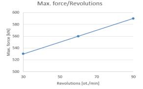
Figure 7. Maximal achieved force with respect to forging rolls revolutions
