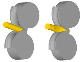
Figure 3. Virtual model of tools for forging rolls with forged part
