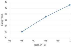
Figure 9. Energy consumption of forging rolls with respect to friction coefficient
