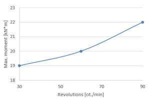
Figure 8. Maximal moment with respect to forging rolls revolutions
