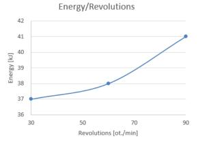
Figure 6. Consumed energy with respect to forging rolls revolutions
