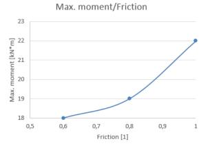
Figure 11. Maximal moment achieved by forging rolls with respect to friction coefficient
