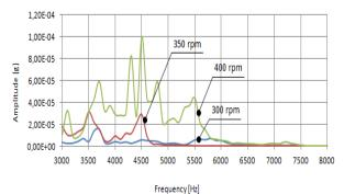
**Figure 6.** Comparison graph of frequency range covers with material removal of 2.7 mm and rotation speed of the head of the milling machine 300, 350 and 400 rpm for processing using the plate-milling machine
