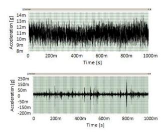
**Figure 3.** Progression of vibration acceleration depending on time and depth of the cut 2.7 and 4.8 mm and spindle rotation speed 300 rpm under processing by a monolith milling machine
