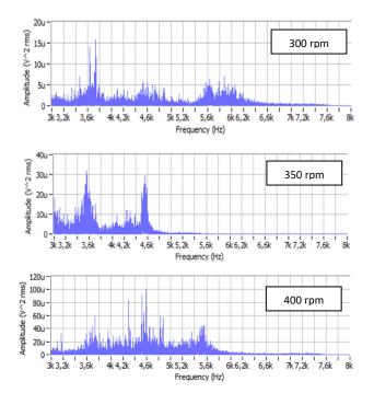
**Figure 4.** Graphic dependency of the vibration acceleration amplitude on frequency with depth of the cut 2.7 mm for processing using the plate milling machine
