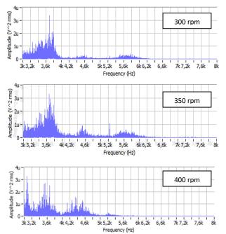
**Figure 5.** Graphic dependency of the vibration acceleration amplitude on frequency with depth of the cut 2.7 mm for processing using the monolith milling machine
