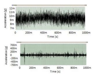
**Figure 2.** Progression of vibration acceleration depending on time and depth of the cut 2.7 and 4.8 mm and spindle rotation speed 300 rpm under processing by a plate milling machine
