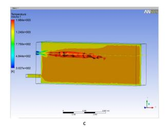
**Figure 3.** Temperature front of the burner and fire-box in combustion a – air composition 1, b - 2, c - 3.
