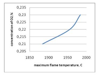
Figure 4. Dependence of O2 concentration on maximum flame temperature
