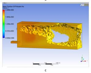
Figure 5. Areas of NO formation above 3 ppm in a – experiment 1, above 30 ppm in b – 2, above 300 ppm c – 3.
