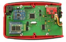
Figure 3. Measurement device prototype version I
