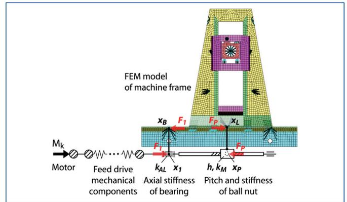
Figure 16. Discrete model of the ball screw feed drive and connection to the machine frame.
