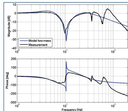
Figure 10. Frequency characteristic of velocity control loop.
