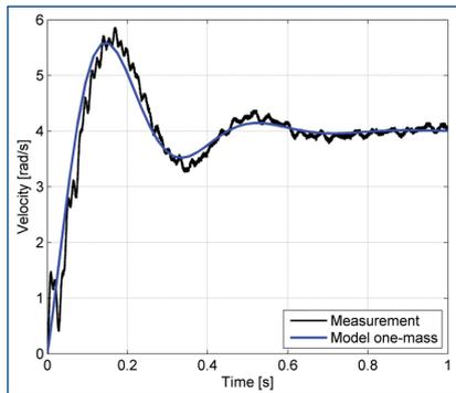
Figure 6. Step response of velocity.
