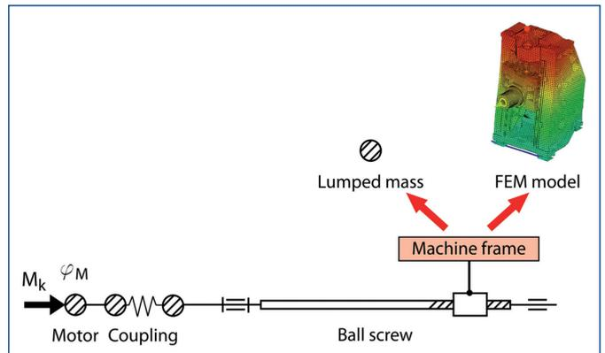
Figure 18. Representation of machine tool movable column by means of lumped mass simplification or FEM model.
