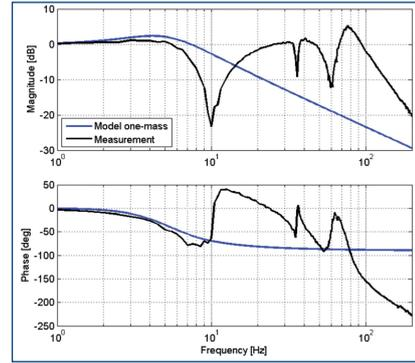
Figure 7. Frequency characteristic of velocity control loop.
