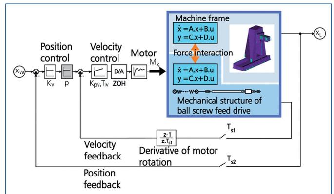
Figure 17. Complex model of servoregulation with ball screw feed drive model coupled with machine frame.
