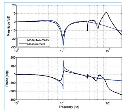
Figure 14. Frequency characteristic of velocity control loop.
