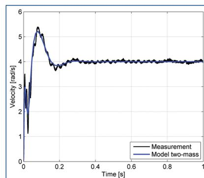
Figure 11. Velocity step response.
