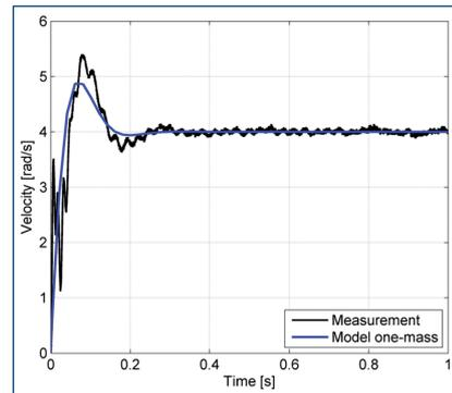
Figure 8. Step response of velocity.
