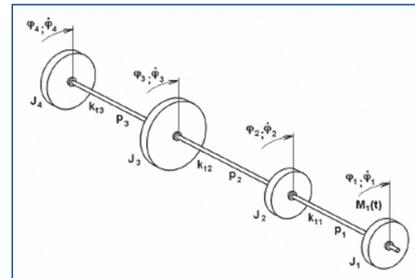
Figure 2. Mechanical structure of the test bed.
