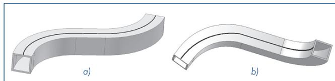
Figure 6. Plane and three-dimensionally bend
