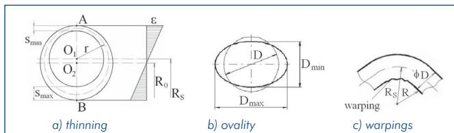
Figure 3. Failures of round tubes after bending
