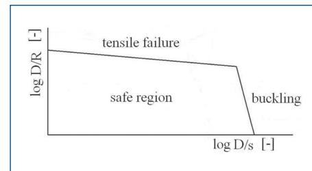
Figure 4. Technological forming limit diagram (TFLD)
