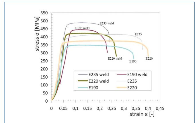
Figure 2. Results of tensile test
