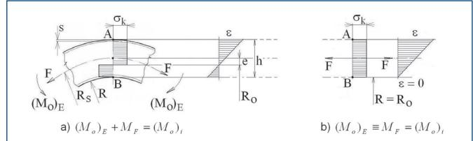
**Figure 12.** Distribution of stresses and engineering strains
