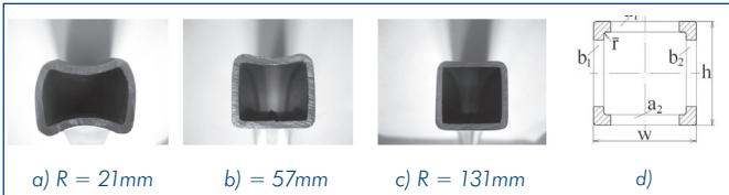
**Figure 9.** Photography of cross-section distortion and denotation of edges
