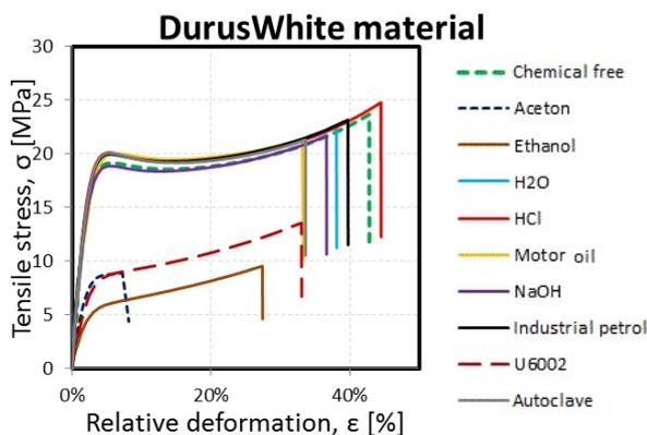
Graph 6. Dependence of the relative deformation on tensile stress for DurusWhite material
