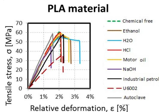
Graph 2. Dependence of the relative deformation on tensile stress for PLA material
