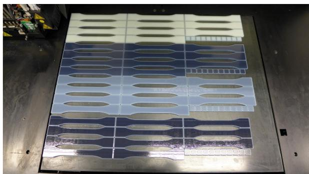
Figure 5. Specimens of photo-polymer materials after printing
