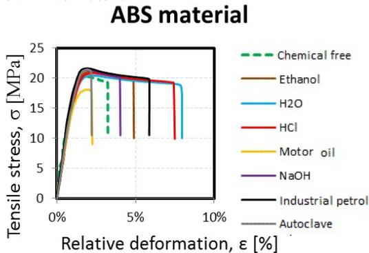
Graph 1. Dependence of the relative deformation on tensile stress for ABS material
