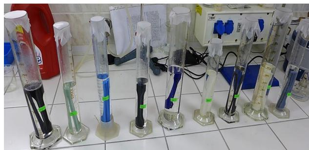
Figure 8. Test specimens immersed in ethanol
