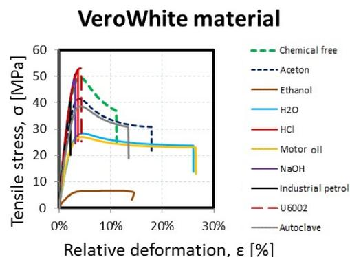
Graph 9. Dependence of the relative deformation on tensile stress for VeroWhite material
