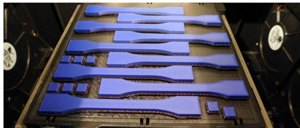
**Figure 4.** Specimens from ABS material after printing.
