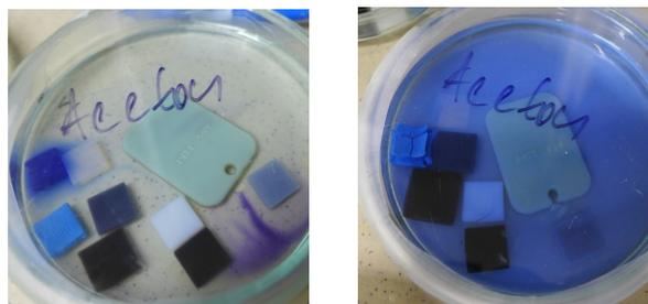
Figure 7. Samples tested in acetone, before and after loading
