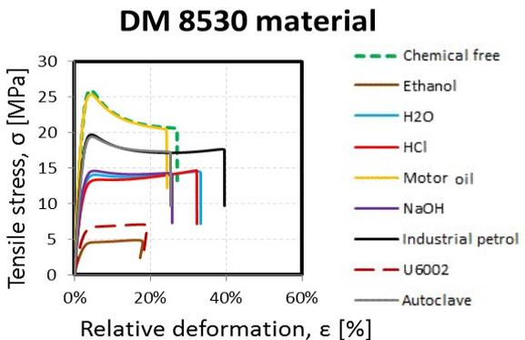
Graph 4. Dependence of the relative deformation on tensile stress for DM 8530 material
