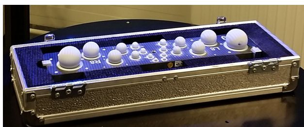
Figure 1. GOM calibration etalon for so called Acceptance Test
