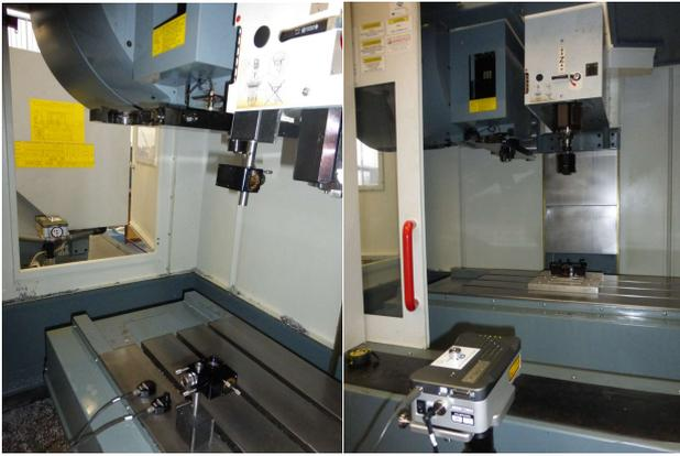
**Figure 4.** Measuring positioning error EZZ with Laser interferometer and volumetric accuracy FRB model with LaserTRACER
