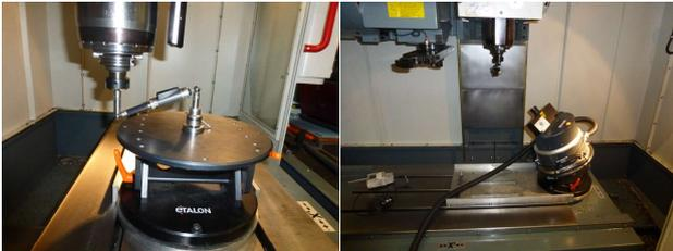
**Figure 5.** Measuring of circularity test with Ballbar and volumetric accuracy RRB model with LaserTRACER
