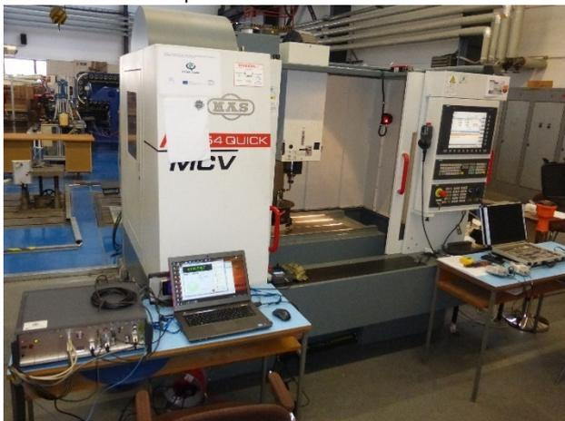
Figure 2. Vertical three-axis machining center MCV 754QUICK
