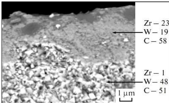
Figure 7. The SEM-image of knife fracture and the ZrN-coating application with elementary composition in different regions marked with arrows, when cutting laminated chipboard
