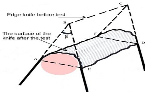
Figure 1. The scheme for calculating the cutting edge wear volume
