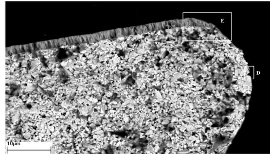
Figure 8. The SEM-image of fracture of worn knife edge with the Mo-N-coating
