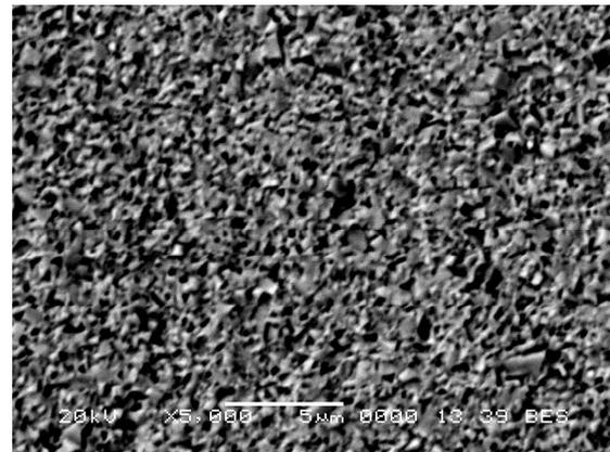
Figure 5. SEM-image of cutting edge surface
