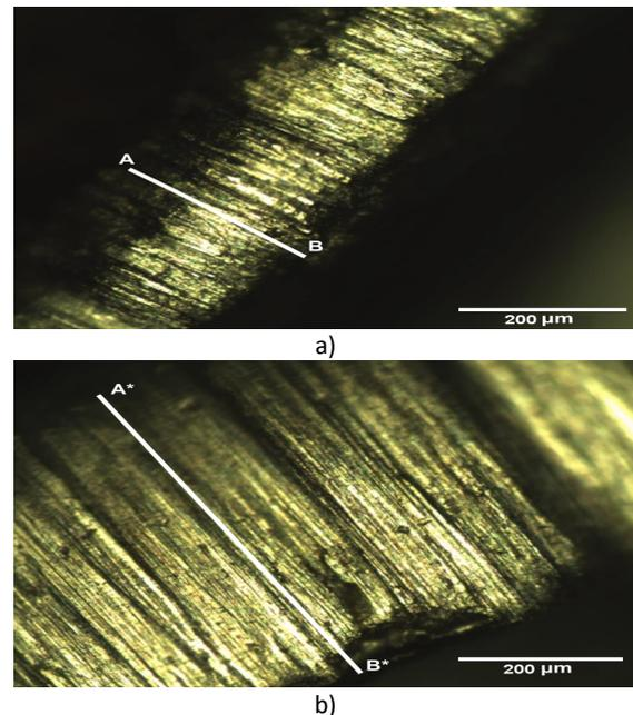
Figure 9. Images of the worn knife edge with the ZrN-Ni-Co-coating (a) and the Ni-Co-coating (b) after milling of laminated chipboard
