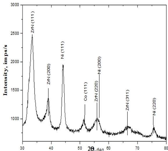
Figure 4. X-rays diagram of ZrN-Ni-Co-coating
