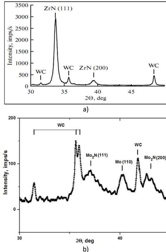
Figure 3. XRD diagrams of the ZrN (a) and Mo-N (b) coatings
