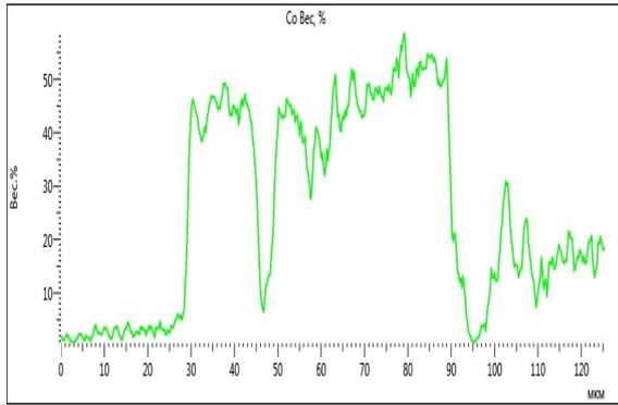
Figure 6. The SEM-image of fracture of cutting edge with the ZrN-Ni-Co-coating (a) and the distribution of Zr (b), Ni (c), Co (d) along the line (a)
