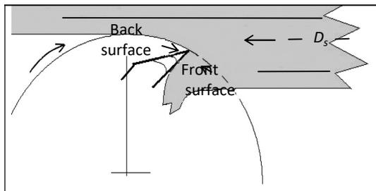
Figure 2. Scheme of interaction of cutting element with processed material
