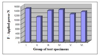
Figure 16. The graph of average measured values of the applied force of the test specimens, type A
