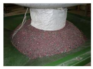
Figure 8. Crushed and sieved plastic waste
