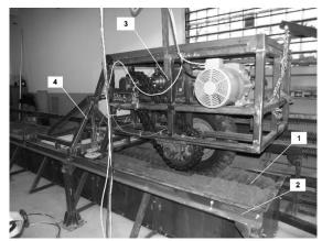
**Figure 1:** Test soil channel 1. The body of the test soil channel with soil, 2. Side routing, 3. Tire support frame, 4. Guide frame
