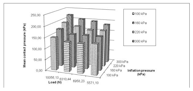
Figure 4. Dependence of the mean tire contact pressure on the load and inflation pressure
