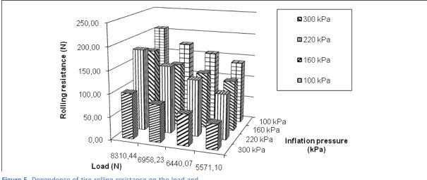
Figure 5. Dependence of tire rolling resistance on the load and inflation pressure
