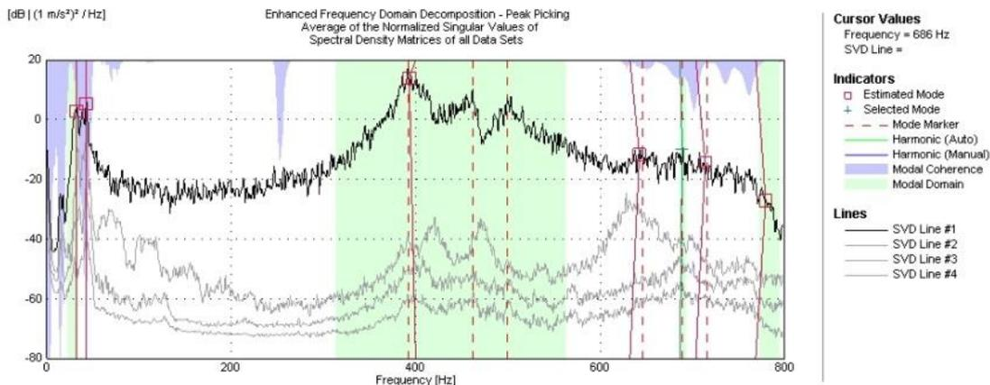
**Figure 15.** Singular values of spectral density matrices estimated by EFDD [Berthold 2016b]
