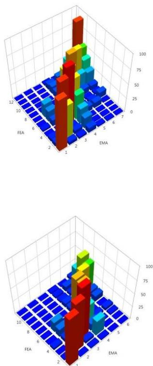
Figure 17 Comparison mode shapes identified by EMA and OMA using the MAC, left: OMA using EFDD, right: OMA using UPC Merged Data Sets
