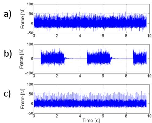
**Figure 14.** Excitation signals in time and frequency domain: (a) random, (b) random burst and (c) random with harmonics [Berthold 2016b].
