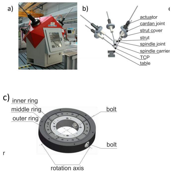
**Figure 11.** Parallel kinematic machine (a) tool with kinematic model of the spindle and the struts (b), cardan joint element (c)
