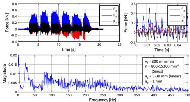
**Figure 10.** Measured cutting forces in time (overview and detail) and frequency domain as result of alternating spindle speed and linear changed immersion [Berthold 2016a].
