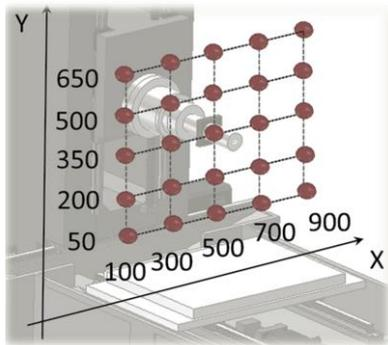
Figure 3. FRF measurement points in the  $X_{NC}$ - $Y_{NC}$ -plane [Putz 2016].
