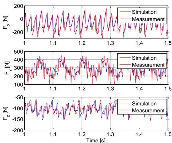
Figure 7. Comparison of calculated and measured cutting forces in time domain [Berthold 2016a].
