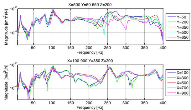
Figure 4. Measured FRF in the x-direction for several machine positions [Putz 2016].
