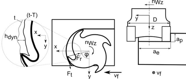
Figure 6. Scheme of the investigated face milling process [Berthold 2016a].
