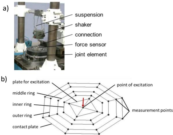
**Figure 12.** Test rig, (a) element mounted in test rig, (b) wire frame model [Berthold 2016b].
