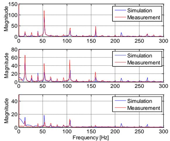
Figure 8. Comparison of calculated and measured cutting forces in frequency domain [Berthold 2016a].
