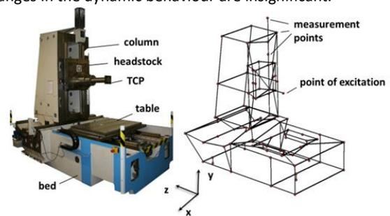
Figure 1. Wire frame model of 3-axis machine tool [Putz 2016].
