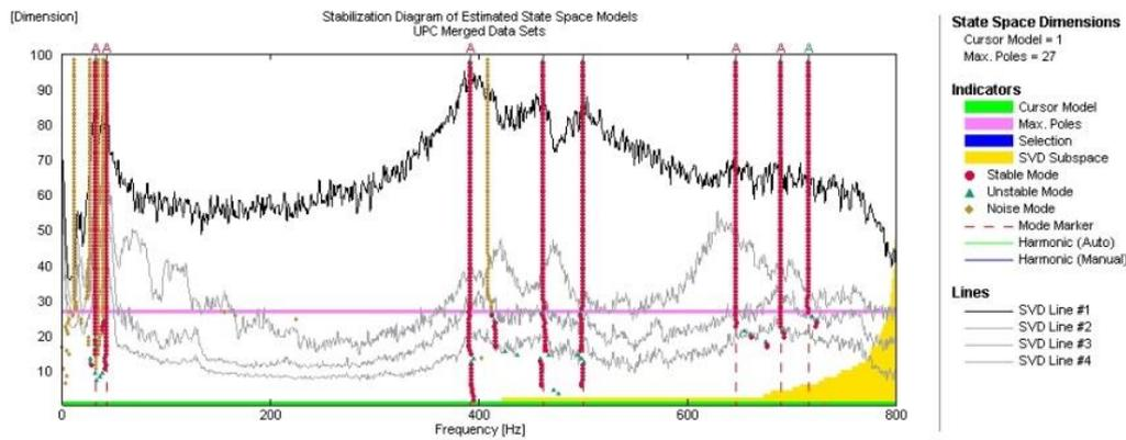
Figure 16 Singular values of spectral density matrices estimated by UPC Merged Data Sets [Berthold 2016b]
