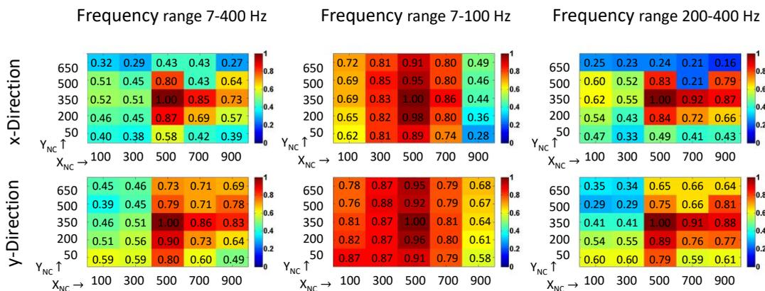
Figure 5. FARC values (also highlighted by colours) in x- and y-direction for different frequency ranges at various machine positions. The reference point for comparison is at  $Z_{NC}=500$ ,  $Y_{NC}=350$ ,  $X_{NC}=200$  [Putz 2016].
