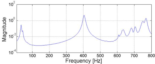
**Figure 13.** Complex Mode Indicator Function (CMIF) for EMA of cardan joint in test rig [Berthold 2016b].
