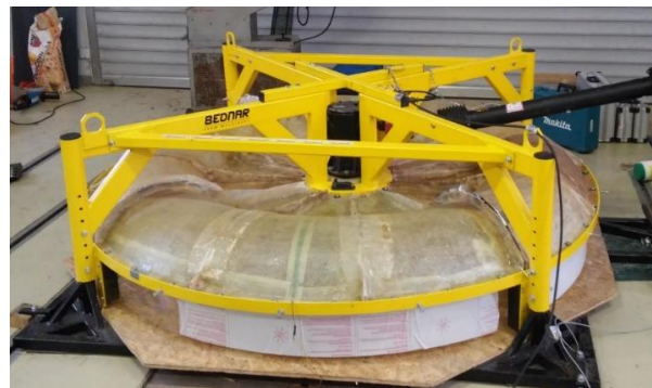
Figure 5. The workspace cover in the shape of "toroid" mounted on the laboratory model
