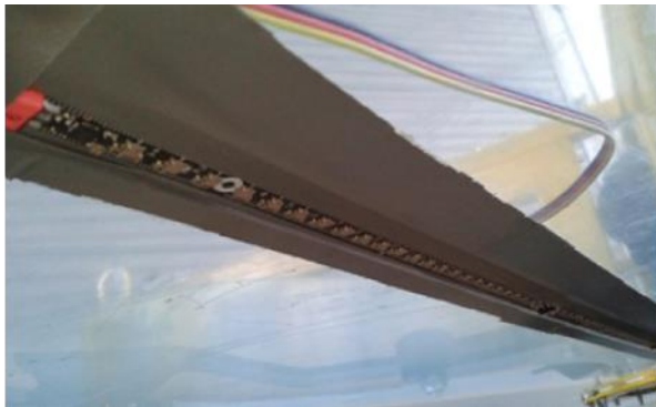
Figure 4. Used pressure sensors, placed on the flat workspace cover
