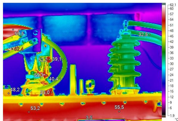
Figure 3. Example of thermogram (biogas plant 1 – transformer object)
