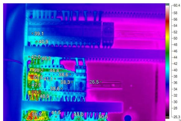
Figure 4. Example of thermogram (biogas plant 2 – machine room)
