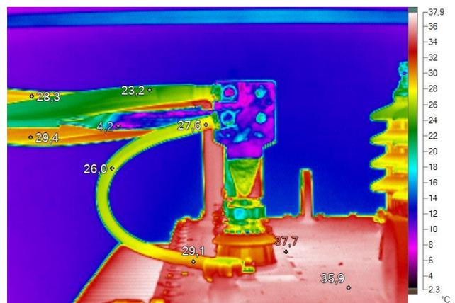
Figure 9. Example of thermogram (biogas plant 3 – transformer object)
