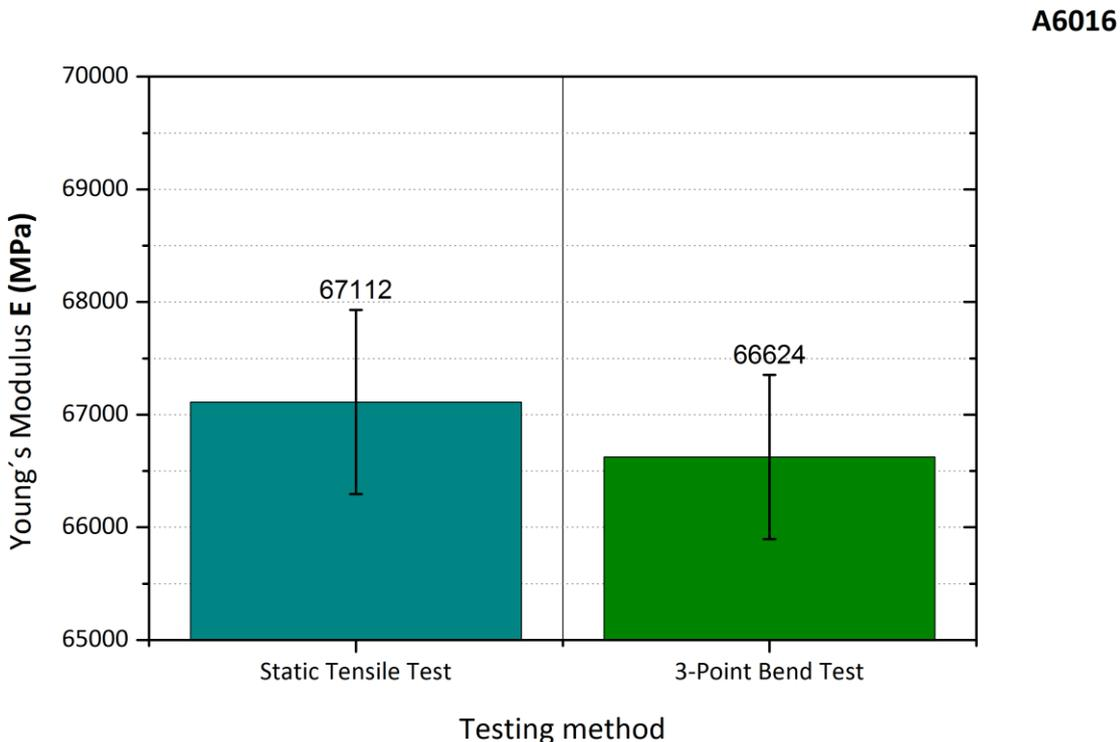
Figure 5. Statistical comparison (by mean and standard deviation) of Young's modulus vs. testing method for A6016
