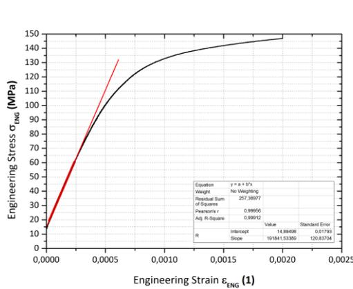
Figure 6. DC06 (static tensile test) – slope of  $\sigma_{ENG}$ -  $\epsilon_{ENG}$  curve
