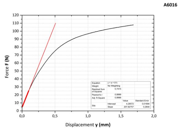
Figure 4. A6016 (3-point bend test) – slope of F - y curve
