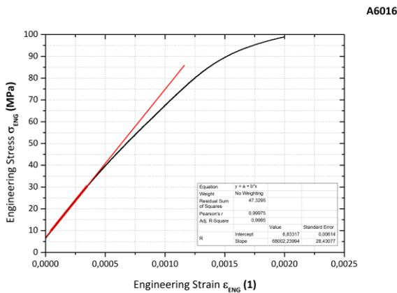
Figure 3. A6016 (static tensile test) – slope of  $\sigma_{ENG} - \epsilon_{ENG}$  CURVE
