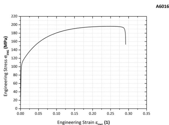
Figure 1. Engineering stress-strain curve for A6016
