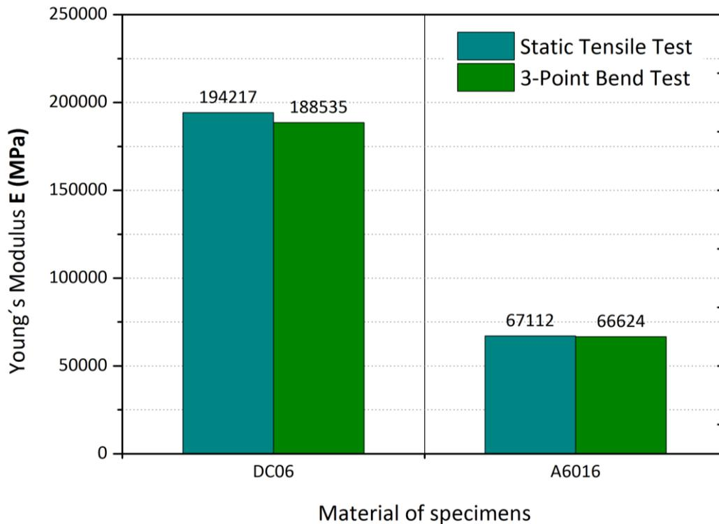
Figure 11. Comparison of Young's modulus in light of used materials and testing methods
