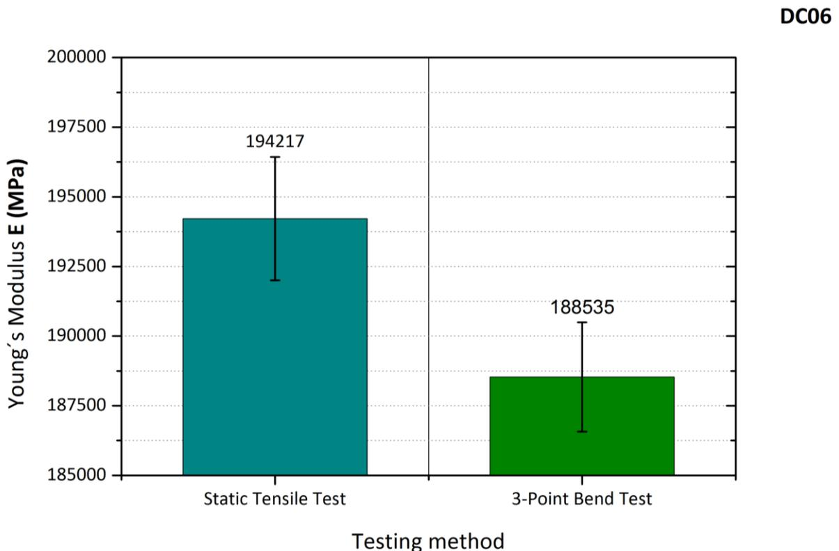
Figure 8. Statistical comparison (by mean and standard deviation) of Young's modulus vs. testing method for DC06
