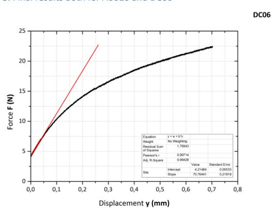
Figure 7. DC06 (3-point bend test) – slope of F - y curve
