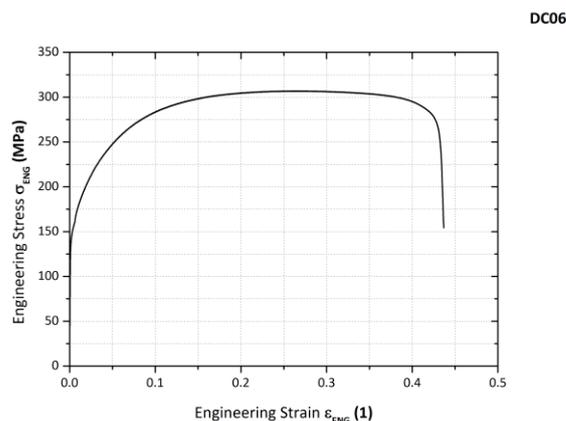
Figure 2. Engineering stress-strain curve for DC06
