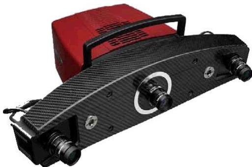
Figure 8. Optical scanner ATOS II 400 [gom.com 2016]
