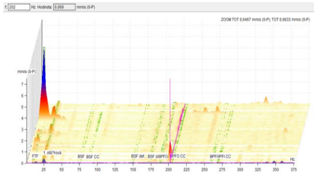
Figure 4. Evolution of the outer ring bearing failure
