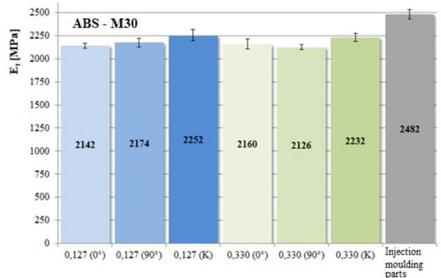
Figure 6. Tensile modulus of ABS-M30 parts: injection moulding vs. 3D print (different fibre orientation and layer thickness)
