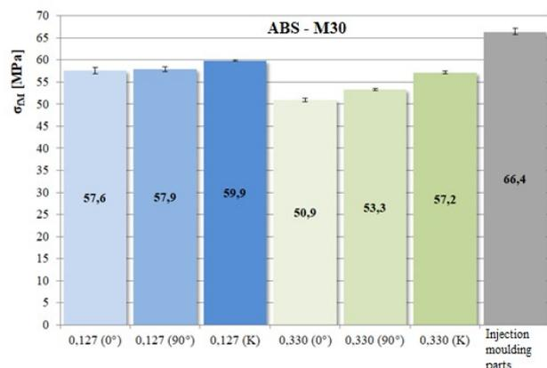
Figure 10. Flexural strength of ABS-M30 parts: injection moulding vs. 3D print (different fibre orientation and layer thickness)
