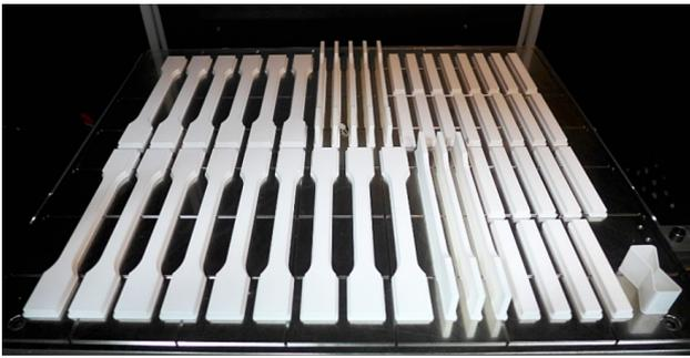
Figure 3. Parts after printing using Fortus 450 with ABS-M30 material.
