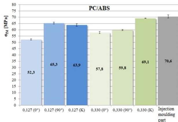
Figure 11. Flexural strength of PC/ABS parts: injection moulding vs. 3D print (different fibre orientation and layer thickness)
