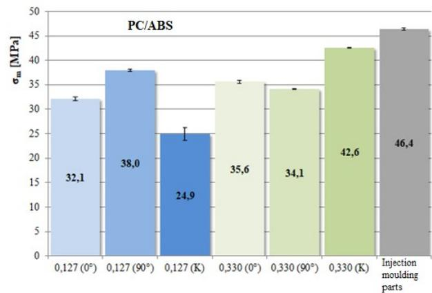
Figure 5. Tensile strength of PC/ABS parts: injection moulding vs. 3D print (different fibre orientation and layer thickness)
