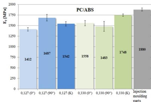
**Figure 13.** Flexural modulus of PC/ABS parts: injection moulding vs. 3D print (different fibre orientation and layer thickness)
