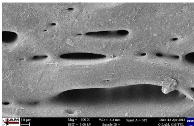
**Figure 17.** Microscopic study of stress cracks on the surface of the injected part made of ABS (acetic acid 99 %, T = 35 °C, t = 60 s).
