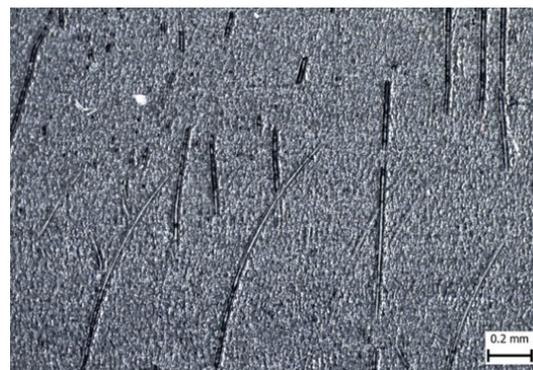
**Figure 16.** Microscopic study of stress cracks on the surface of the injected part made of PC/ABS (acetic acid 99 %,  $T = 35^\circ\text{C}$ ,  $t = 120\text{ s}$ ).
