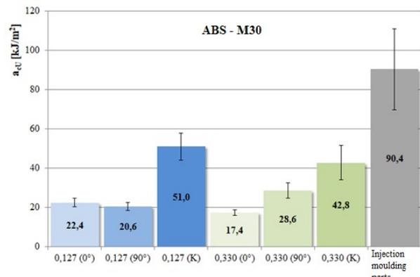
**Figure 14.** Impact strength of ABS parts: injection moulding vs. 3D print (different fibre orientation and layer thickness)
