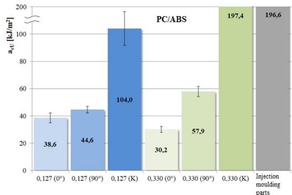
**Figure 15.** Impact strength of PC/ABS parts: injection moulding vs. 3D print (different fibre orientation and layer thickness)
