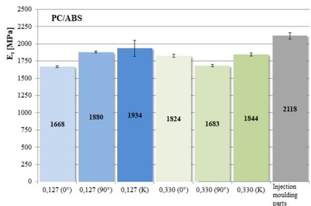
Figure 7. Tensile modulus of PC/ABS parts: injection moulding vs. 3D print (different fibre orientation and layer thickness)
