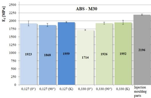
**Figure 12.** Flexural modulus of ABS parts: injection moulding vs. 3D print (different fibre orientation and layer thickness)
