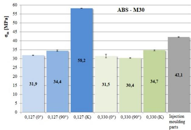
Figure 4. Tensile strength of ABS-M30 parts: injection moulding vs. 3D print (different fibre orientation and layer thickness)
