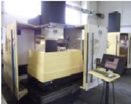
Figure 2. CNC electroerosion device Agietron IMPACT 3 of Agie Charmilles
