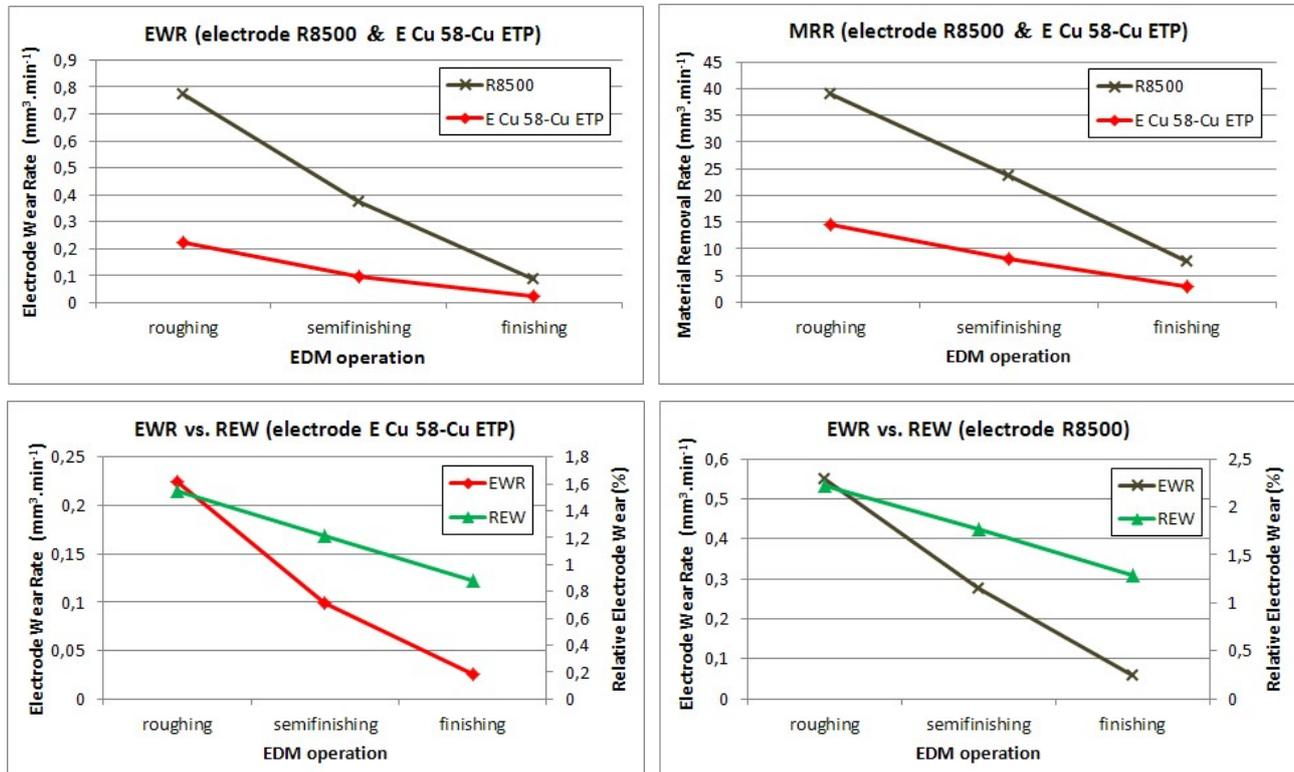
**Figure 4.** Dependence of the monitored output parameters EWR, REW and MRR to the type of operation (roughing, semifinishing and finishing) EDM the steel EN 90MnCrV8 using the shape of the electrodes E Cu 58-Cu ETP and R8500
