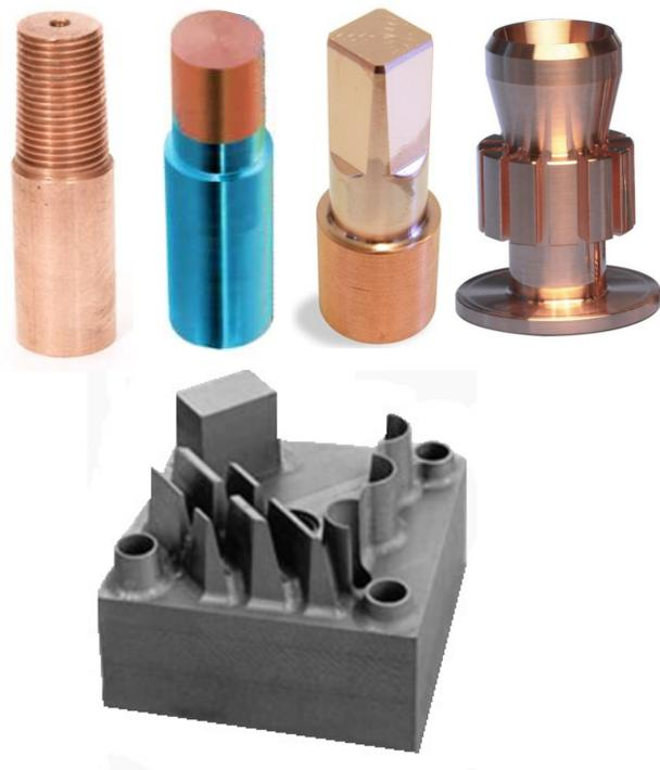
Figure 1. Electrode shapes for EDM prone to wear
