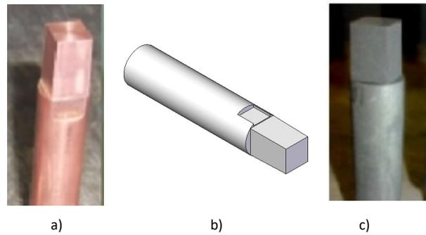
Figure 3. Cu and graphite shaped tool electrode used in the experiment
