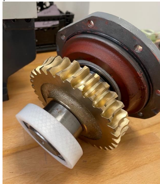
Figure 4. Damping inserts made of NYLON PA12 material installed in a worm gearbox
