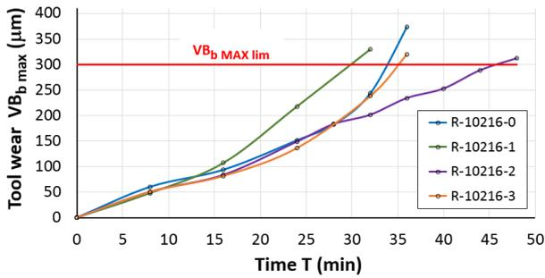
Figure 7. Graphical comparison of average  $VB_{b\max}$  wear characteristics for all tested tools when Inconel 718 conventional milling with cutting conditions:  $v_c = 40 \text{ m}\cdot\text{min}^{-1}$ ,  $f_z = 0.06 \text{ mm}$ ,  $a_e = 0.5 \text{ mm}$ ,  $a_p = 4 \text{ mm}$
