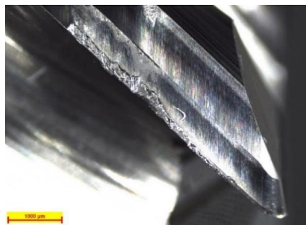
Figure 6. Typical tool wear during conventional roughing of Inconel 718
