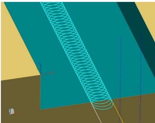
Figure 3. Proposed trochoidal toolpath for milling
