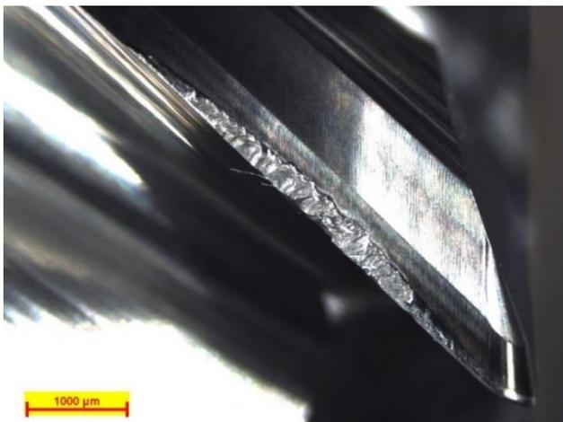
Figure 8. Typical tool wear during trochoidal milling of Inconel 718
