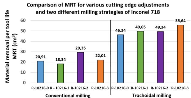
Figure 10. Comparison of volume of material removed per tool life (MRT) for various cutting edge adjustments and two different milling strategies
