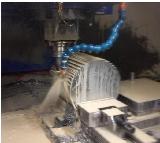
Figure 4. Clamped workpiece on the machine tool prepared for milling
