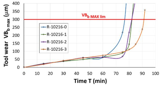
Figure 9. Graphical comparison of average  $VB_{b\max}$  wear characteristics for all tested tools when Inconel 718 trochoidal milling with cutting conditions:  $v_c = 40 \text{ m}\cdot\text{min}^{-1}$ ,  $f_z = 0.06 \text{ mm}$ ,  $a_e = 0.5 \text{ mm}$ ,  $a_p = 4 \text{ mm}$
