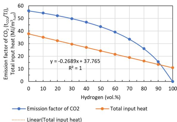
Figure 8. Evolution of the emission factor depending on the addition of hydrogen to natural gas
