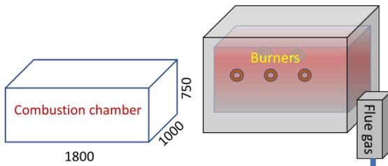
Figure 4. Dimension of the combustion chamber [Kizek 2021]
