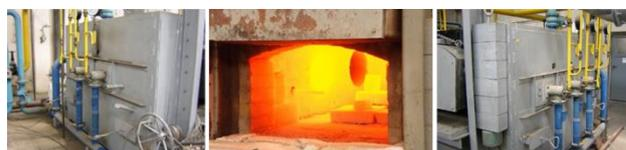
Figure 1. Heating chamber furnace with heat input 5x100 kW
