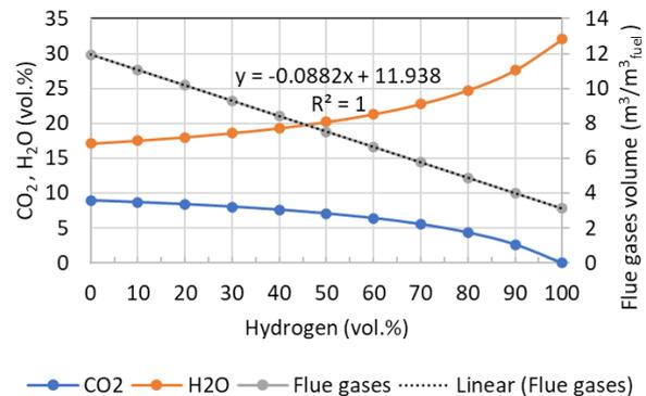
Figure 6. Course of the content of  $\text{CO}_2$  and  $\text{H}_2\text{O}$  flue gas components and the amount of actual flue gas depending on the addition of hydrogen to natural gas
