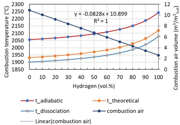
Figure 5. Course of combustion temperatures and amount of combustion air depending on the concentration of hydrogen in the natural gas
