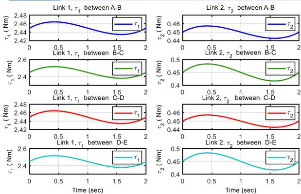
**Figure 20.** Torques  $\tau_1$  and  $\tau_2$  of the joint, where  $m_1=0.4$  kg,  $m_2=0.3$  kg
