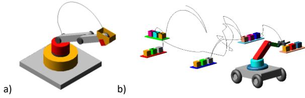
**Figure 2.** Two-link robotic arm with trajectory of end point in MSC Adams software a) on a fixed arm, b) on a mobile arm
