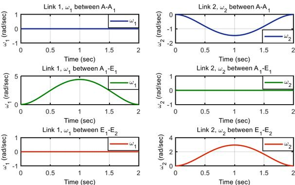
**Figure 15. Angular velocities  $\omega_1$  and  $\omega_2$  of the end point movement from point A-A<sub>1</sub>, A<sub>1</sub>-E<sub>1</sub>, E<sub>1</sub>-E<sub>2</sub>**
