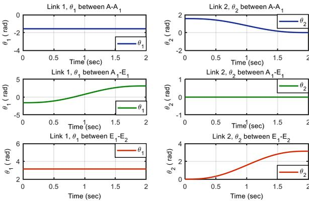
**Figure 14. Rotation angle  $\theta_1$  and  $\theta_2$  of the end point movement from point A-A<sub>1</sub>, A<sub>1</sub>-E<sub>1</sub>, E<sub>1</sub>-E<sub>2</sub>**
