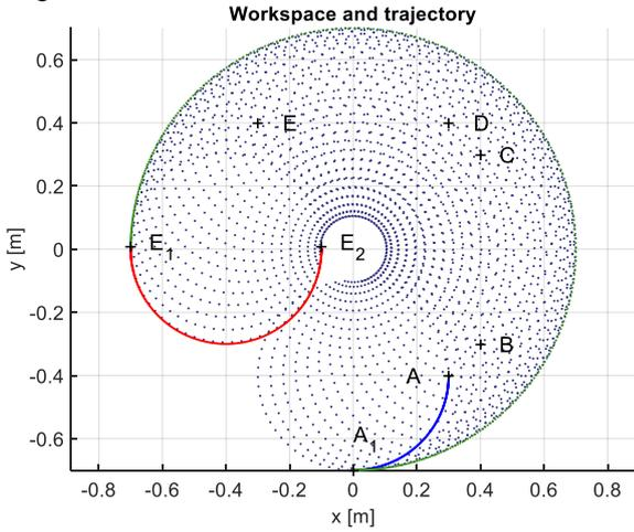
**Figure 13. Coordinates x-y for different combinations of angles  $\theta_1$  and  $\theta_2$  for angle constraint  $-90^\circ \leq \theta_1 \leq 180^\circ$ , angle constraint  $-175^\circ \leq \theta_2 \leq 175^\circ$  and trajectory from point A-A<sub>1</sub>, A<sub>1</sub>-E<sub>1</sub>, E<sub>1</sub>-E<sub>2</sub>**
