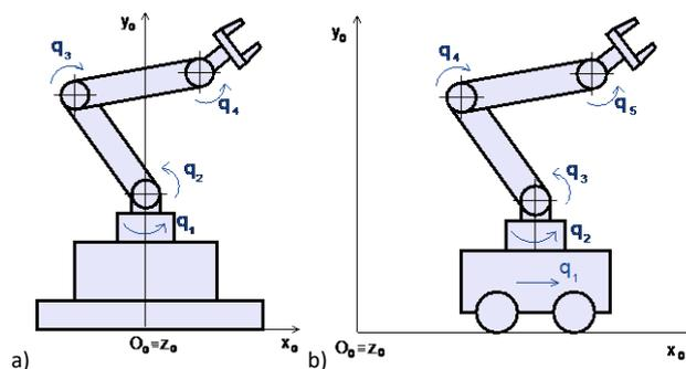
Figure 1. Two-link robotic arm a) on a fixed base, b) on a mobile chassis
