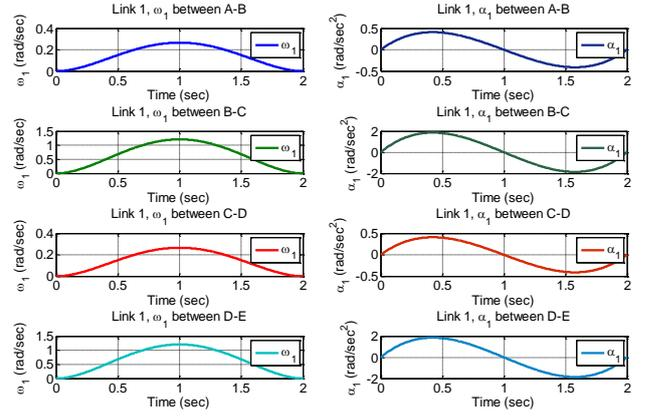
**Figure 11.** Angular velocity  $\omega_1$  and angular acceleration  $\alpha_1$  of the Link 1 (arm 1) of movement from initial point A to final point B (A-B), B-C, C-D, D-E
