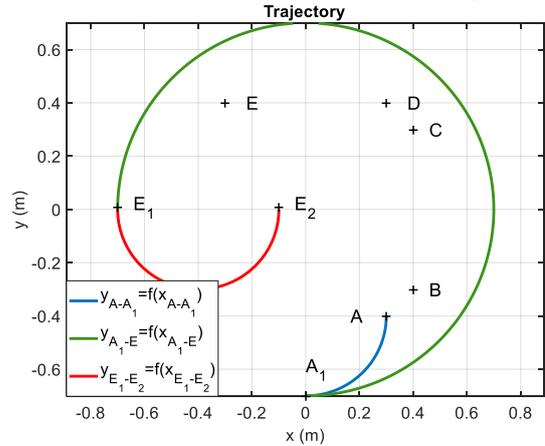
**Figure 12.** Trajectory of the end point movement from point A- $A_1$ ,  $A_1$ - $E_1$ ,  $E_1$ - $E_2$
