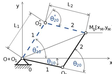
**Figure 5.** Mechanical system with 2 degrees of freedom and rotation angles  $\theta_{10}$  a  $\theta_{20}$  for initial position of the arm and rotation angles  $\theta_{10}^*$  a  $\theta_{20}^*$  for final position of the end point
