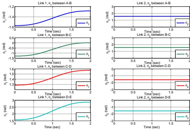
**Figure 10.** Rotation angles  $\theta_1$  and  $\theta_2$  of the Link 1 and Link 2 of movement from initial point A to final point B (A-B), B-C, C-D, D-E
