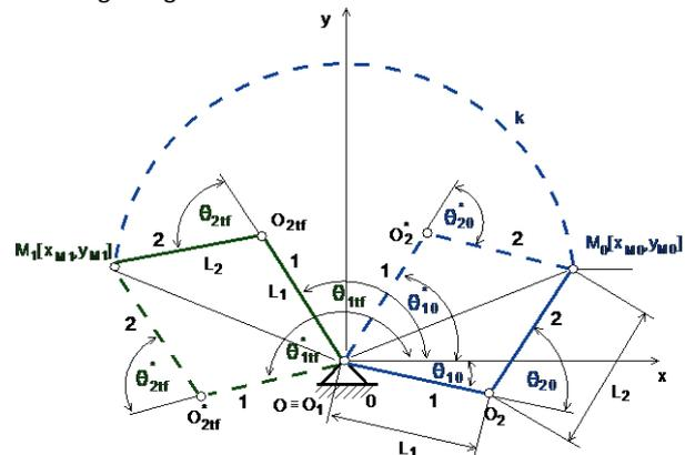
**Figure 6.** Initial and final position of the point M
