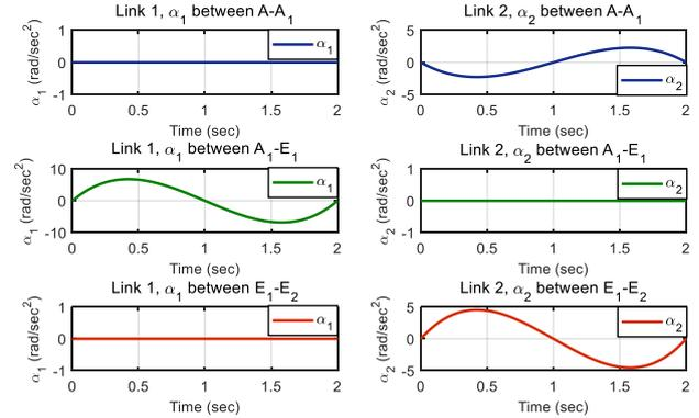
**Figure 16. Angular accelerations  $\alpha_1$  and  $\alpha_2$  of the end point movement from point A-A<sub>1</sub>, A<sub>1</sub>-E<sub>1</sub>, E<sub>1</sub>-E<sub>2</sub>**
