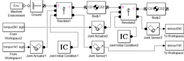
**Figure 19.** SimMechanics block diagram for determining the angular motion produced by torques  $\tau_1$  and  $\tau_2$  in joints of member 1 and member 2
