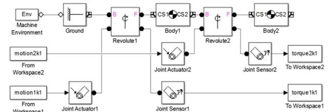
**Figure 18. SimMechanics block diagram for determining torques  $\tau_1$  and  $\tau_2$  in joint of member 1 (Link 1) and member 2 (Link 2)**
