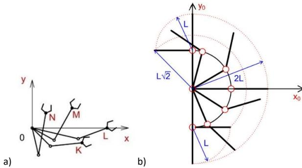
**Figure 3.** Two-link robotic arm a) in working positions K, L, M, N, b) in various working positions
