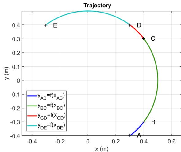
**Figure 8.** Trajectory components of the end point movement from initial position in point A to position in point B and from point B to point C, C-D and D-E
