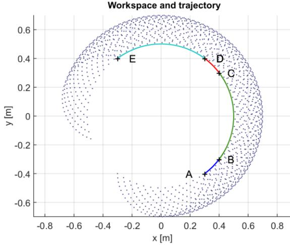
**Figure 9.** Coordinates x-y for different combinations of  $\theta_1$  ( $-90^\circ \leq \theta_1 \leq 165^\circ$ ) and  $\theta_2$  ( $-90^\circ \leq \theta_2 \leq 90^\circ$ ) and trajectory of the end point movement from point A-B, B-C, C-D, D-E
