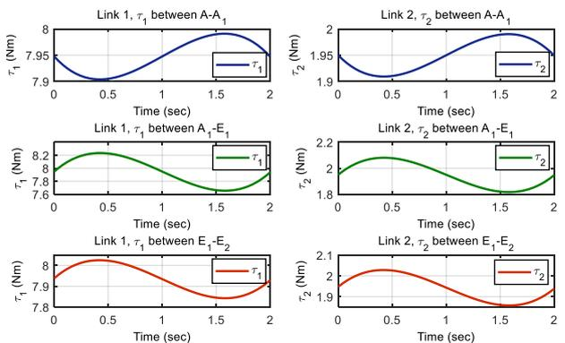
**Figure 23.** The torques  $\tau_1$ ,  $\tau_2$  in joint,  $m_1=0.4$  kg,  $m_2=1.3$  kg
