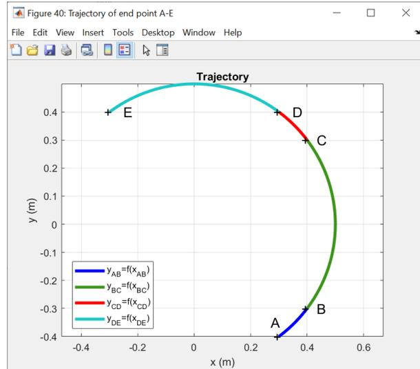
**Figure 7.** Trajectory components of the end point movement from initial position in point A to position in point B and from point B to point C, C-D and D-E
