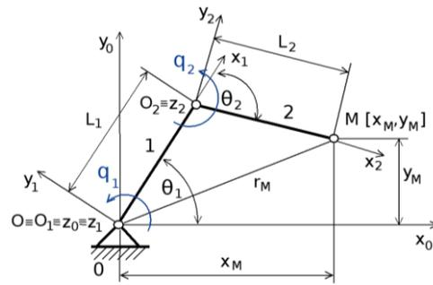
**Figure 4.** Mechanical system with 2 degrees of freedom and generalized coordinates  $q_1$  and  $q_2$  ( $q_1 = \theta_1$  a  $q_2 = \theta_2$ )
