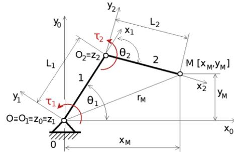
**Figure 17. Two-link robotic arm with joint torques  $\tau_1$  and  $\tau_2$**
