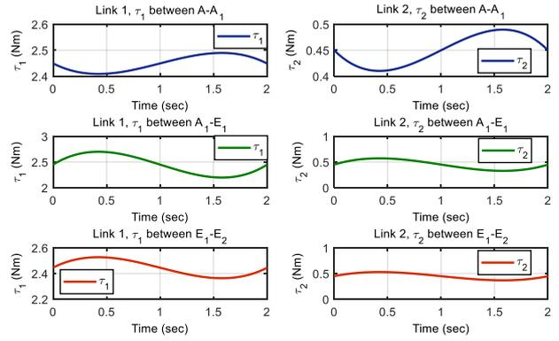
**Figure 21.** Torques  $\tau_1$  and  $\tau_2$  of the joint, where  $m_1=0.4$ kg,  $m_2=0.3$ kg
