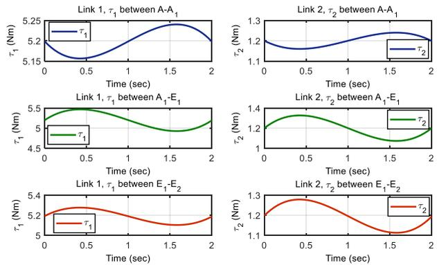
**Figure 22.** The torques  $\tau_1$ ,  $\tau_2$  in joint,  $m_1=0.4$  kg,  $m_2=0.8$  kg
