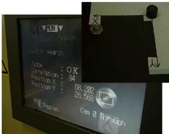
Figure 3. Output from the selected camera system
