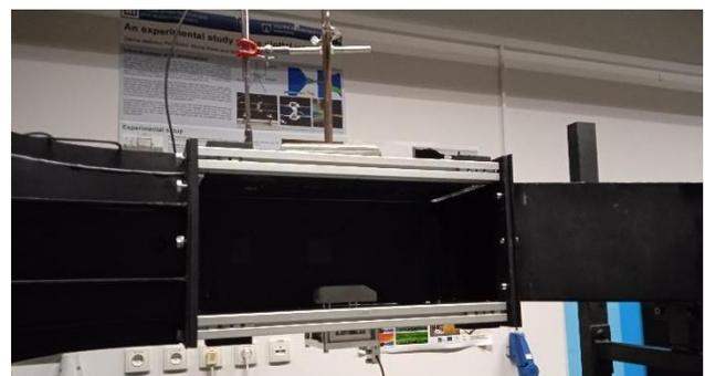
Figure 6 Wind tunnel with the mounted model and measuring equipment
