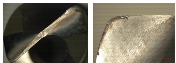
Fig. 8: Outer corner wear of drill 16N
