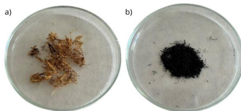
Figure 1. Samples of coconut fibers before (a) and after pyrolysis process (b)
