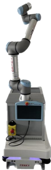
Figure 1. Combination of the collaborative robot UR5e and the mobile tugger MiR100 [own elaboration 2025]
