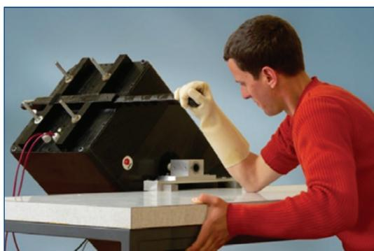
Figure 5. Representation of the Arm Wrestling Robot [Kovacs 2007]
