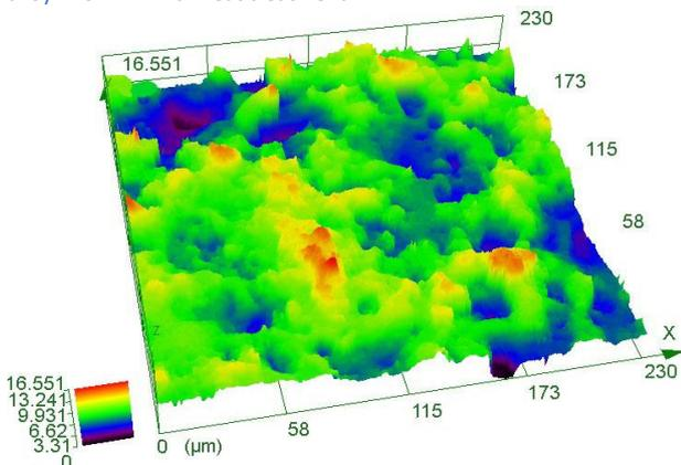
**Figure 5.** 3D picture of the sample 2 made of titanium alloy Ti-6Al-4V with heat treatment, magnified 1200x,  $T_{on}=8 \mu s$ ,  $T_{off}=55 \mu s$ , current=25 A
