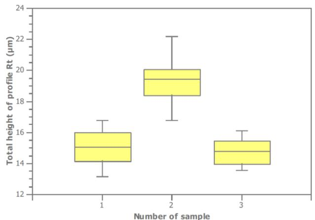
**Graph 5.** Total height of profile Rt of the samples made of steel X210Cr12 with the type of heat treatment 4
