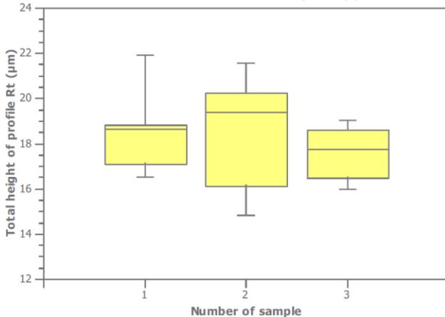
**Graph 3.** Total height of profile Rt of the samples made of steel X210Cr12 with the type of heat treatment 2
