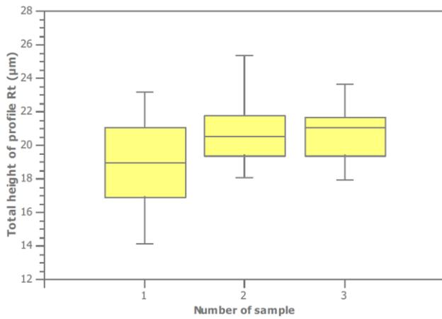
**Graph 6.** Total height of profile Rt of the samples made of titanium alloy Ti-6Al-4V without heat treatment
