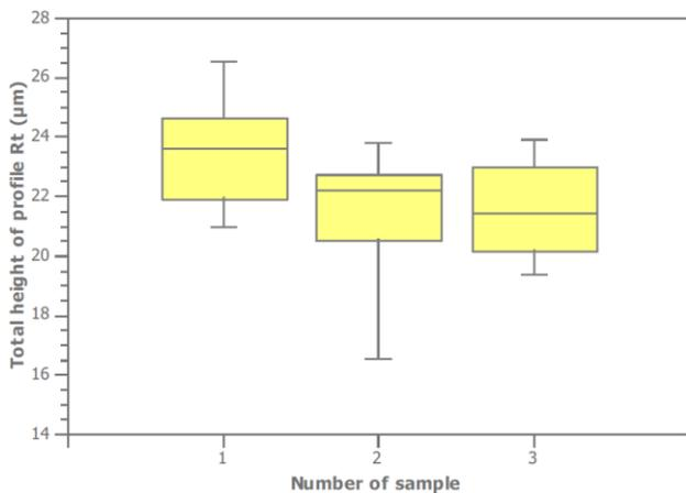
**Graph 7.** Total height of profile Rt of the samples made of titanium alloy Ti-6Al-4V with heat treatment
