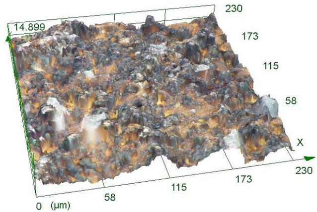
**Figure 4.** 3D picture of the sample 2 made of steel X210Cr12 with the heat treatment 2, magnified 1 200x,  $T_{on}=8 \mu\text{s}$ ,  $T_{off}=55 \mu\text{s}$ , current=25 A
