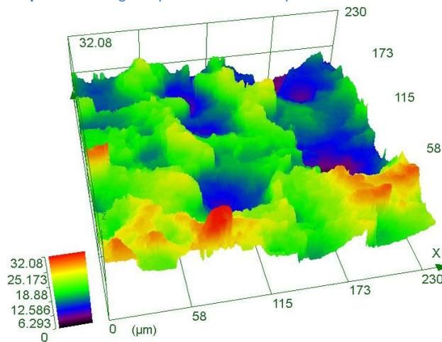
**Figure 1.** 3D picture of the sample 2 made of Al 99.5 magnified 1,200x,  $T_{on}=8 \mu$ s,  $T_{off}=55 \mu$ s, current=25 A
