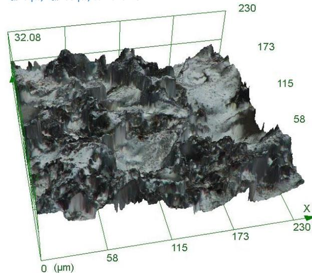
**Figure 2.** 3D picture of the sample 2 made of Al 99.5 magnified 1,200x,  $T_{on}=8 \mu$ s,  $T_{off}=55 \mu$ s, current=25 A
