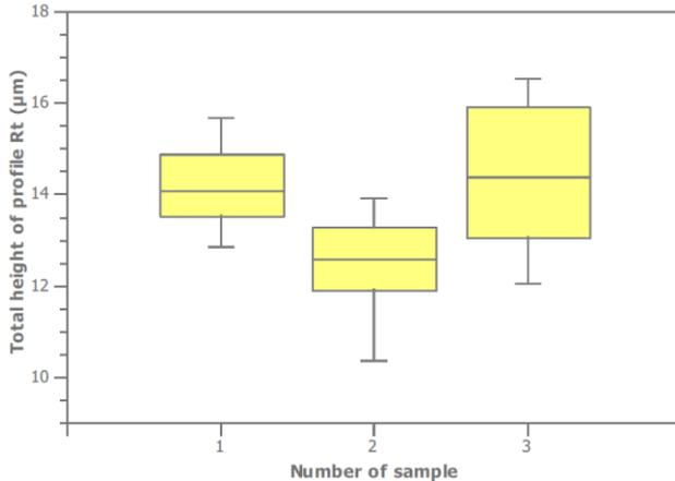
**Graph 2.** Total height of profile Rt of the samples made of steel X210Cr12 with the type of heat treatment 1
