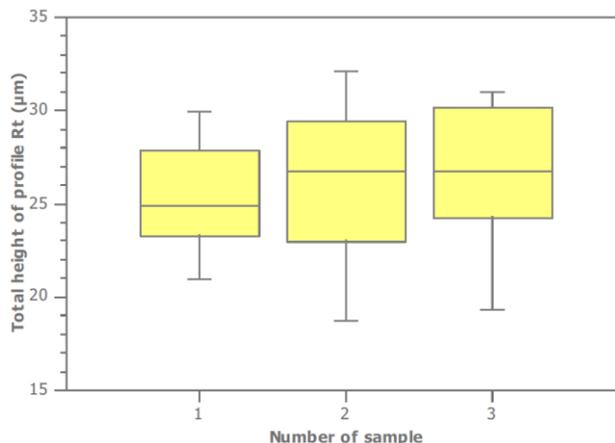
**Graph 1.** Total height of profile  $R_t$  of the samples made of Al 99.5
