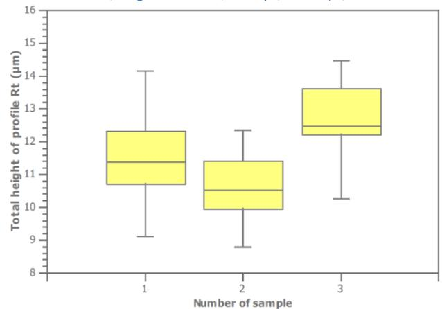
**Graph 4.** Total height of profile Rt of the samples made of steel X210Cr12 with the type of heat treatment 3
