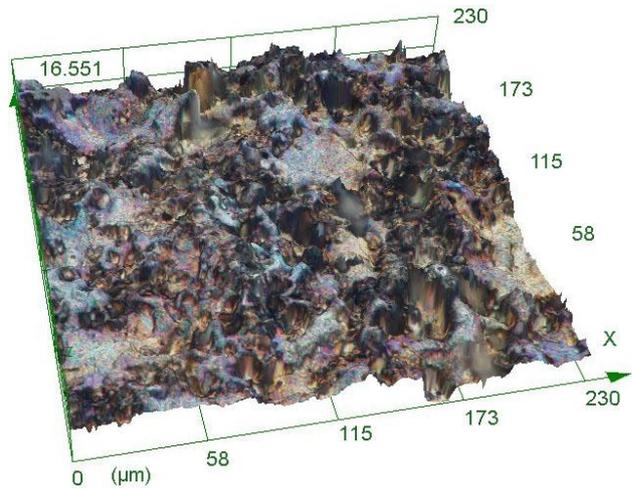
**Figure 6.** 3D picture of the sample 2 made of titanium alloy Ti-6Al-4V with heat treatment, magnified 1200x,  $T_{on}=8 \mu s$ ,  $T_{off}=55 \mu s$ , current=25 A
