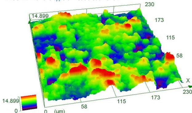
**Figure 3.** 3D picture of the sample 2 made of steel X210Cr12 with the heat treatment 2, magnified 1 200x,  $T_{on}=8 \mu\text{s}$ ,  $T_{off}=55 \mu\text{s}$ , current=25 A
