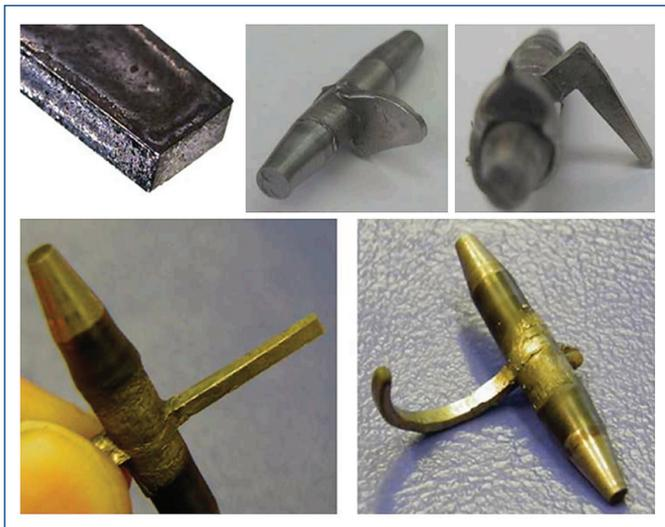
Figure 11. Example demonstration products produced by mini-thixoforming
