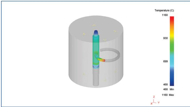
**Figure 7.** Results for initial temperature of the tools 20 °C: material of the tools – steel X210Cr12
