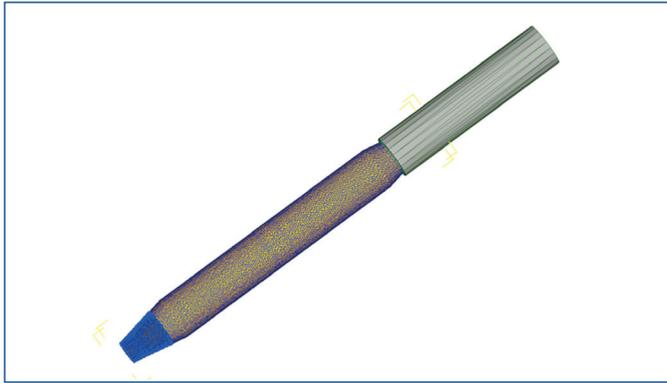
Figure 3. Overview of FEM mesh: Contact of test specimen and die at the beginning of the simulation before forming is blue labeled
