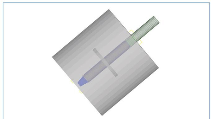
Figure 2. Complete computational model: die, mandrel and the test specimen
