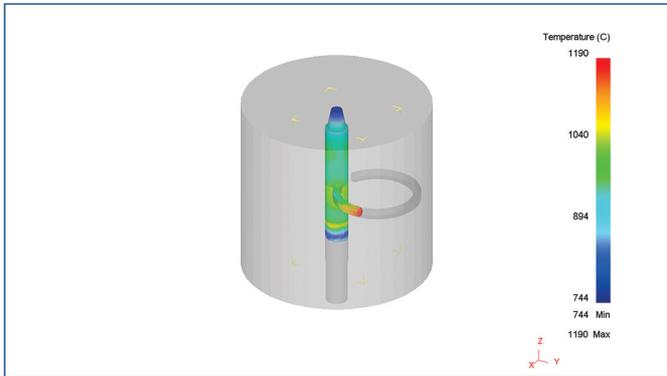
**Figure 8.** Results for initial temperature of the tool 300 °C: material of the tools – Titan Grade 5
