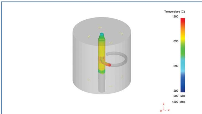
**Figure 9.** Results for initial temperature of the tool 300 °C: material of the tools – steel X210Cr12
