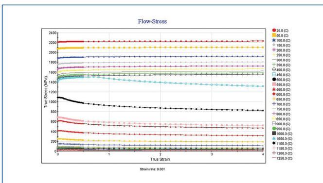
Figure 5. Flow stress of the material CPM15V calculated by JMatPro
