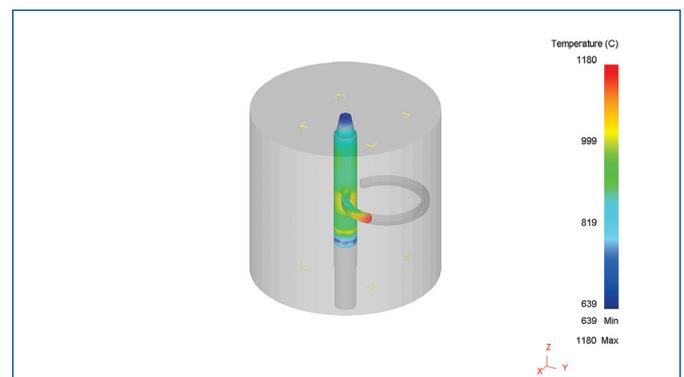
Figure 6. Results for initial temperature of the tools 20 °C: material of the tools – Titan Grade 5
