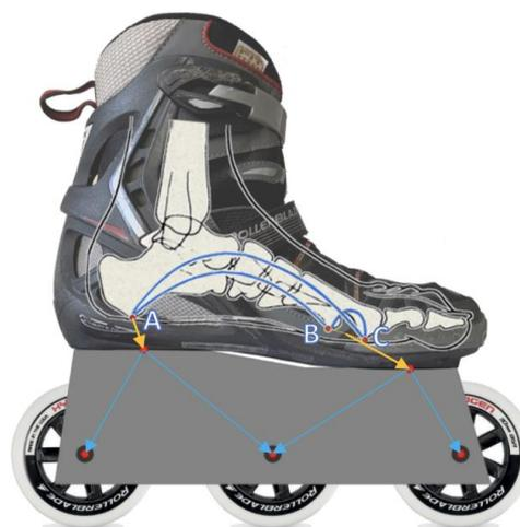
Fig. 3: Scheme of load distribution of skater weight on the frame.
