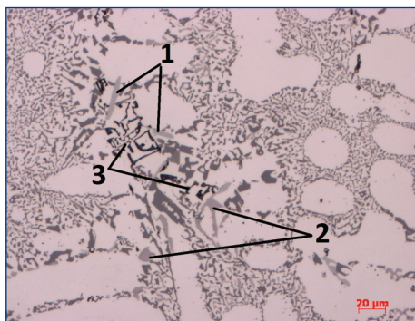
Figure 1. AlSr3.5 modified sample – characteristic intermetallic phases at grain boundaries, 200x, 1 – phase of iron, probably \beta\text{-Al}_5\text{FeSi} , 2 – phase of iron and manganese, probably \text{Al}_{15}(\text{FeMn})_3\text{Si}_2 , 3 – phase of magnesium \text{Mg}_2\text{Si}
