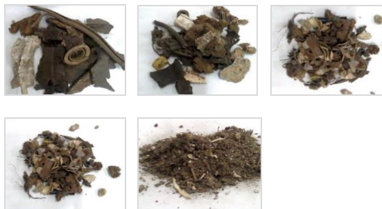
Figure 2. Granulometric classes a) + 50 mm; b) - 50 + 25 mm; c) - 25 + 15 mm; d) - 15 + 10 mm; e) - 10 + 0 mm.
