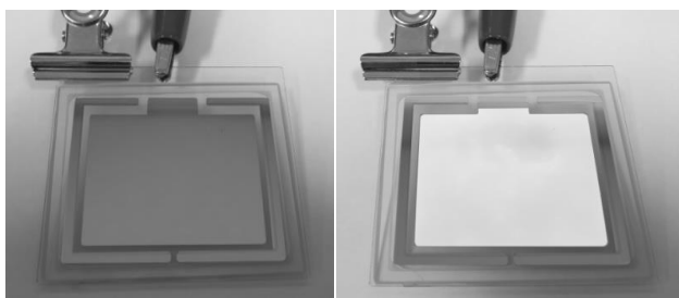
Figure 12. An appearance of the trial manufactured panel with an emission area of 34mm x 30 mm (Left: Power off state, Right: Power on state)
