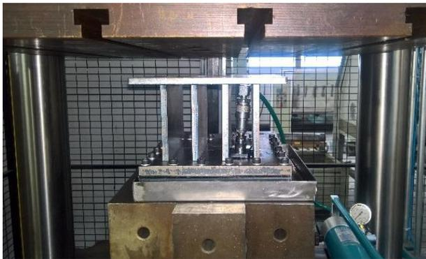
Figure 13. Hydroforming device in a hydraulic press
