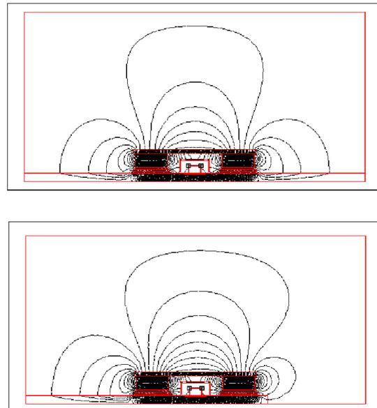
Figure 13: A model of magnetic field lines in the case of an infinite (up) and finite (down) rope
