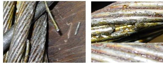
Figure 5b. A photo of artificially created internal defects
