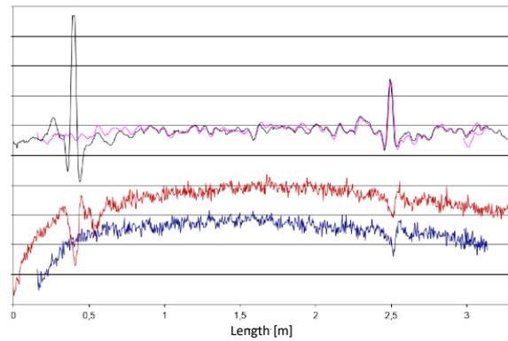
Figure 9: A record of reference sample R1 from defectoscope MID-3 (up) and REMA (down)
