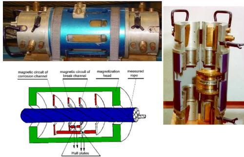
Figure 7. The REMA magnetic defectoscope and its model configuration used during experimental analysis
