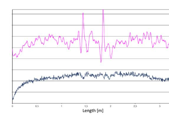
Figure 12: A record of reference sample R4 from defectoscope MID-3 (up) and REMA (down)
