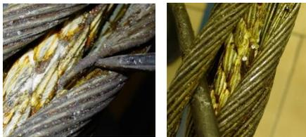
Figure 3. A photo of reference sample R1 and a photo of the artificially created internal damage
