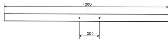
Figure 6: An illustration of reference sample R4, showing artificially created internal defects
