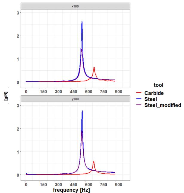
Figure 7. FRF Amplitude X and Y axis
