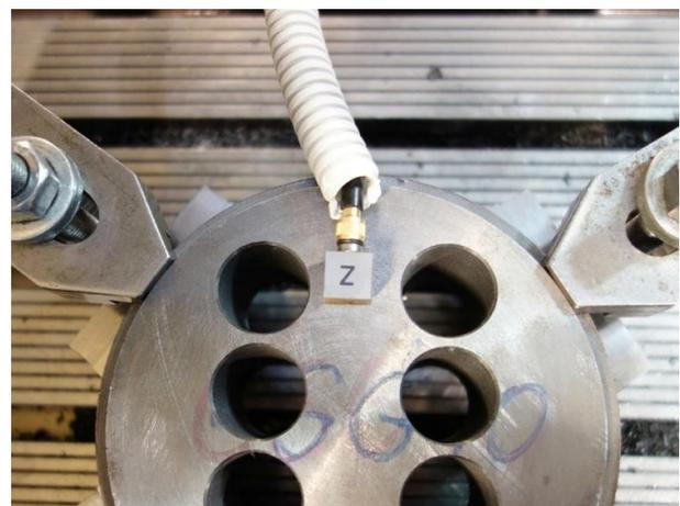
Figure 8. Dynamic experiment- accelerometer position
