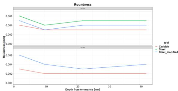
Figure 17. Geometry quality of hole- all designs
