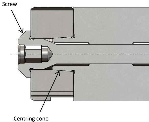
Figure 1. Clamping system
