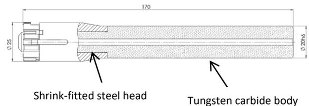
Figure 4. Solid carbide design
