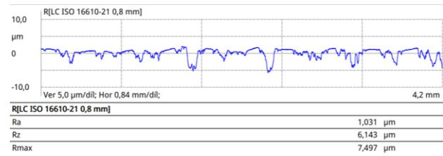
Figure 15. Roughness profile  $v_c=350\text{m/min}$  cemented carbide toolbar
