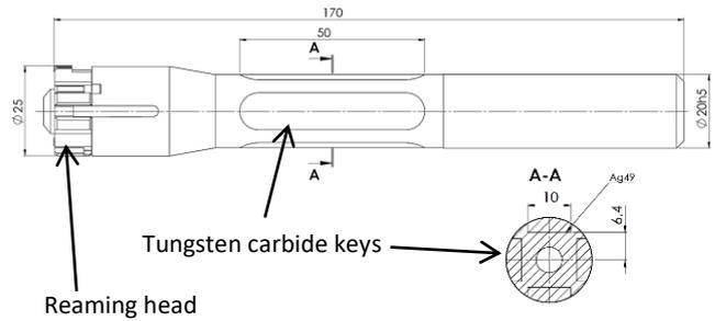
Figure 3. Modified steel toolbar
