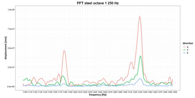
Figure 10. Steel tool bar FFT detail 20th band
