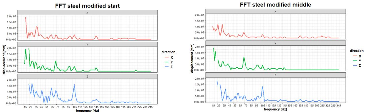
Figure 11. FFT comparison modified steel tool bar
