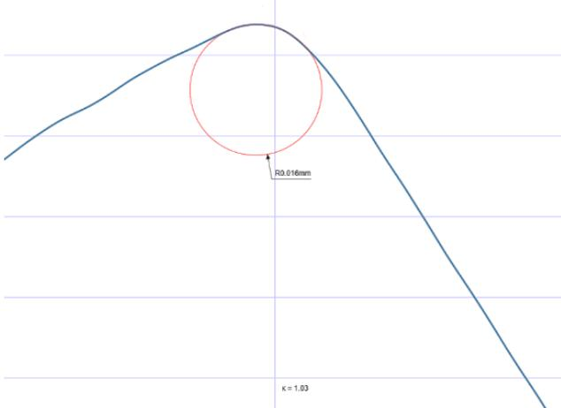
Figure 5. Tool micro geometry
