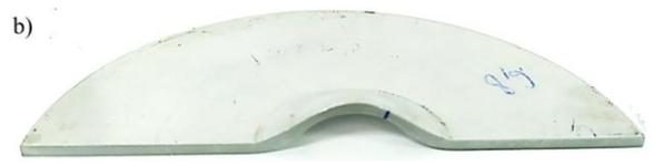
**Figure 7.** Necking position for samples with depth of indentation EI1 =6.7mm(a) and EI2=6.8mm (b)
