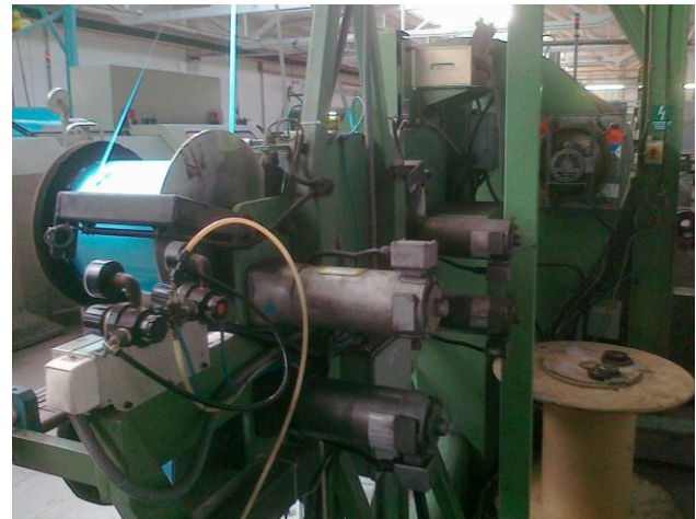
Figure 1. Automated cable winder with drive head diagnostics using vibration analysis methods
