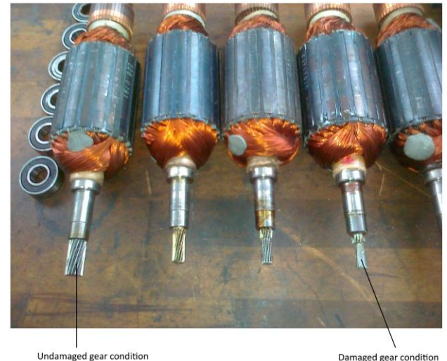
Figure 8. Types of damage to the rotor gear pinion
