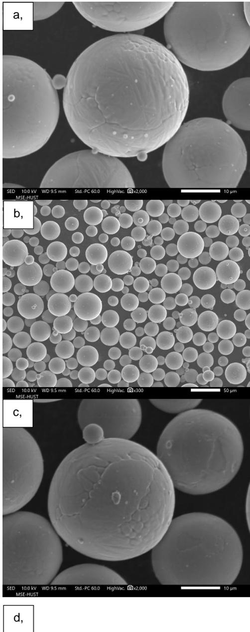
**Figure 1.** SEM micrographs of: a, b) virgin Ti-6Al-4V powder and c, d) printed Ti-6Al-4V powder
