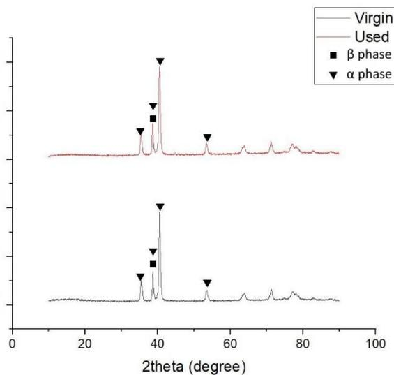
**Figure 5.** XRD patterns of used and virgin Ti6Al4V metal powder.
