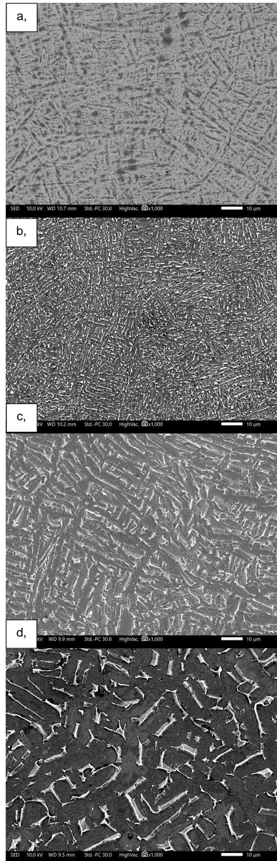
**Figure 2.** SEM micrographs of: a) as-built b) 850 °C annealed c) 950 °C annealed and d) 1050 °C annealed sample
