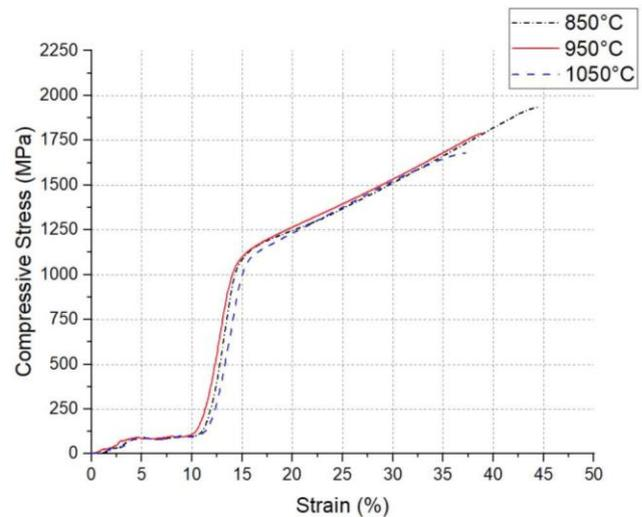
Figure 4. Stress-strain curve for Compression Test Result
