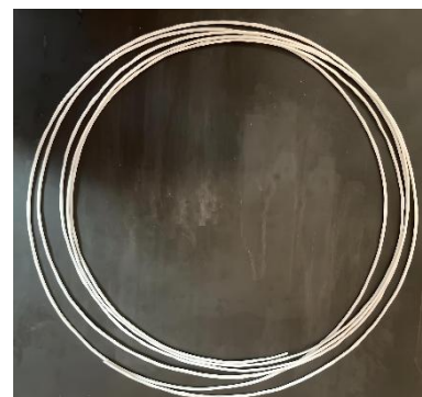
Figure 2a. Filament morphology under 270° C extrusion
